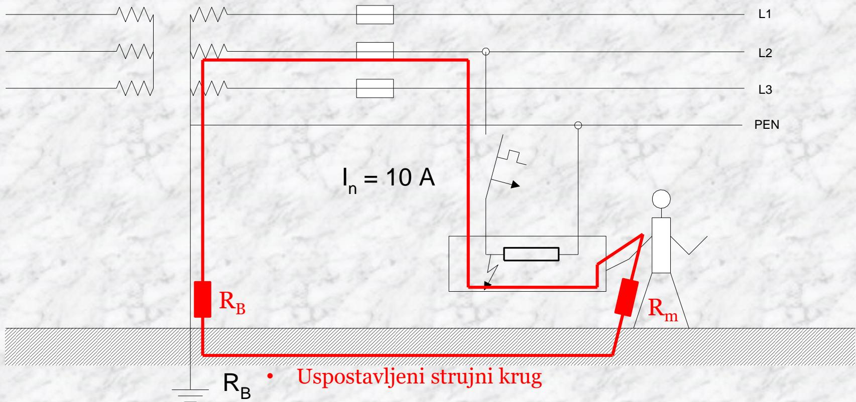
$$R_B = 2 \Omega, U_1 = 230 \text{ V}, R_m = 1000 \Omega, R_A = 5 \Omega,$$
